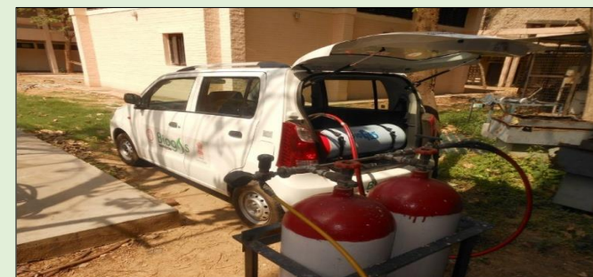
Biogas dispensing system at IIT Delhi
